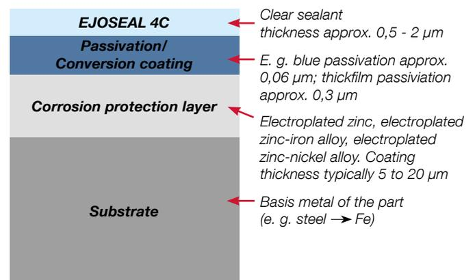
General structure of electroplated zinc or zinc alloy coating with EJOSEAL 4C
