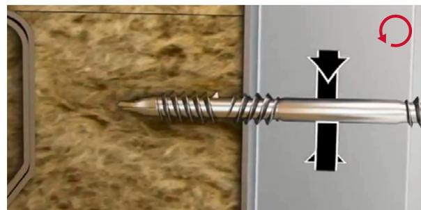
Installing through outer sheet (**anti-clockwise – left**)
