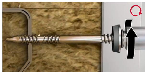
Drilling cassette substructure (**clockwise – right**)
